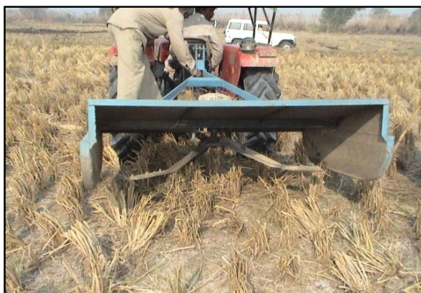
Fig. 1. Shrub master in operation in field.
