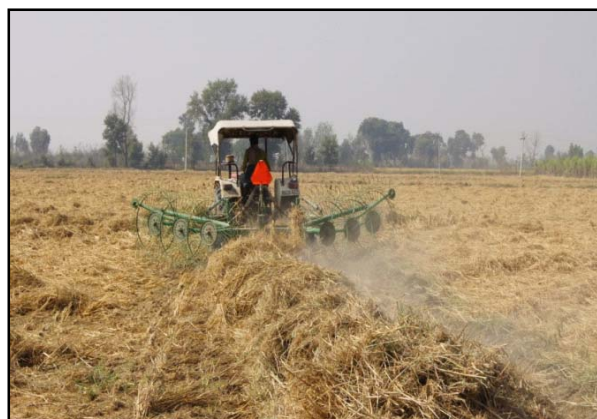
Fig. 2. Hay rake in operation in field.
