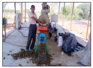
(Source: http://www.igfri.res.in/images-new/fmpht-feed-palleting.jpg) Fig. 4. Compact feed pelleting machine.
