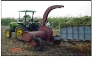
(Source:http://ecoursesonline.iasri.res.in/pluginfile.php/2529/ mod\_page/content/1/Module%204%20Lesson%207%20Fig.7.3.jpg) Fig. 1. Tractor operated flail fodder harvester-chaffer-loader.
